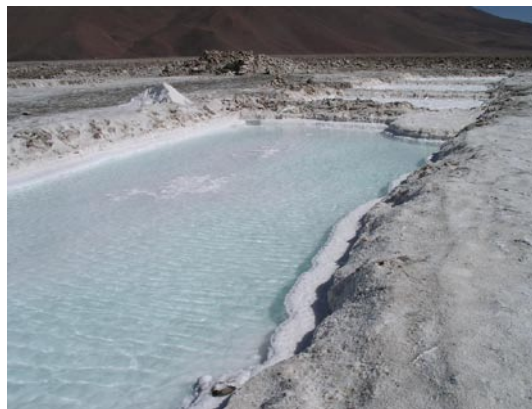
Pilot evaporation pond for concentrating brine to 10,000 ppm of Lithium.
