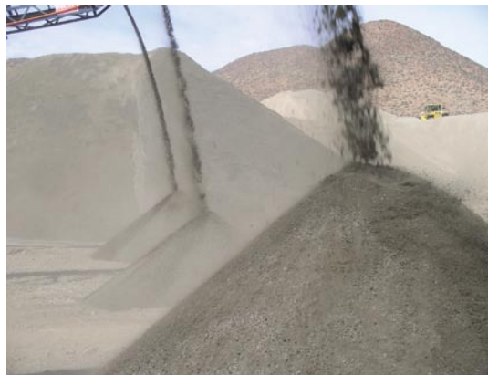
64.5% Fe iron ore on conveyors after being separated by magnetic drums
