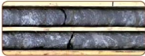
Example of Magnetite in Veins from Mariposa Total iron grade: 60% max, 30% average
