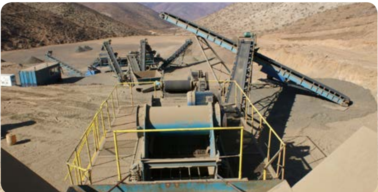
Figure 4: Crushing and processing plant where the live production test on Soberana run of mine was performed in July. Equipment owned by Minera MACS S.A.
